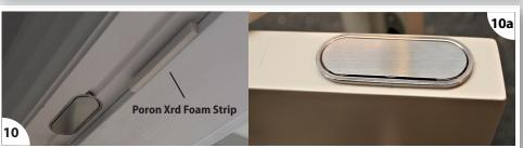
10. Once the desired magnetic holding strength has been achieved, affix the **SELF ADHESIVE S/STEEL COVERPLATES** to the magnetic face(s) of the ASSEMBLIES as shown, to protect the magnets from corrosion and for a more attractive 'concealed fix' finish. (10, 10a)
