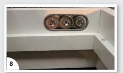
8. Insert **DOOR JAMB MAGNETIC ASSEMBLY** into head jamb and secure with 2 x screws provided.
